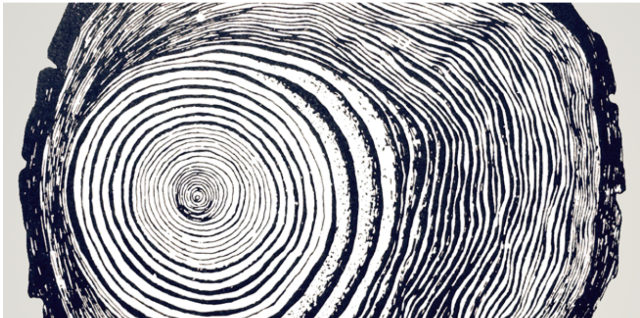
Figure 1: Cross-section of softwood (1)
